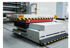
Unloading car for turret winder
