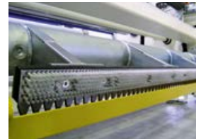
Automatic reel change system TAC shortly before cutting
