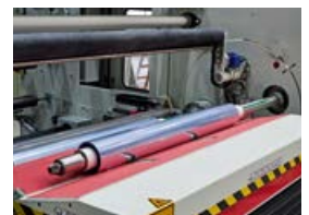
Integrated shaft extraction device in the ATW turret winder
