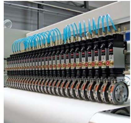
Automatic slitting system
